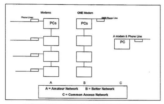
System A is an amateur implementation in that the redundant use of multiple pieces of equipment does not provide a more robust network.
